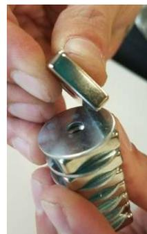
Carefully "peel off" a magnet and washer from the stack stored in the protective tube.
