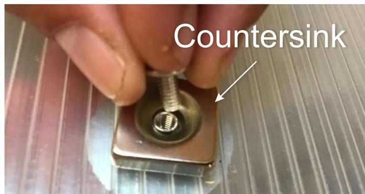
Countersink side of magnet faces wire on coop. Install magnets in all remaining holes on panel.
